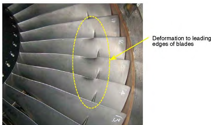
Figure 9: Birdstrike damage to right engine fan blade on Boeing 767, 3 October 2006
